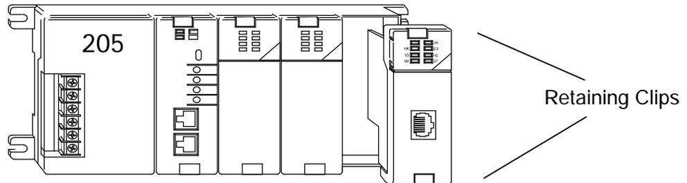
To install the ERM module, line up the module's printed circuit board with the grooves in the base and push the module until it is flush with face of the DL205 base power supply. If you feel more than moderate resistance when you push the module into the base, the circuit board may not be aligned with the grooves in the base. When the module is firmly seated in the slot, depress the top and bottom retaining clips to lock the module in place.
