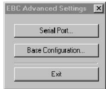
When you click on the Base Configuration button (top of page) the *H4-EBC Base Configuration* screen pops up, as shown below. The H2-EBC and the T1H-EBC are self-configuring and do not require this step.
