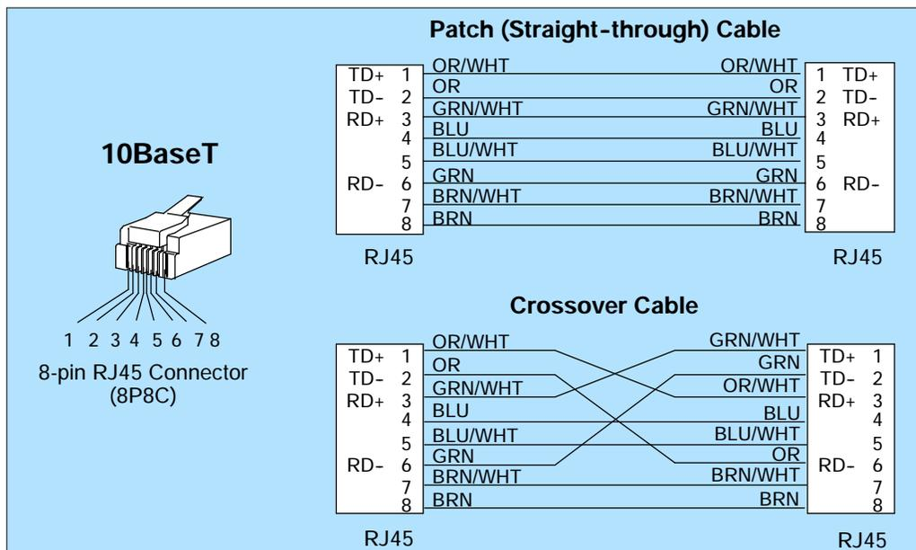
This diagram illustrates the standard wire positions in the RJ45 connector. We recommend all ERM 10BaseT cables to be **Category 5**, UTP cable.
