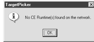
Acknowledge this message by clicking OK, and the “Think &Do ESP CE Station Selection” window will open. If you have not already done so, install the WinPLC and connect power to the DL205 base. See pages 1-4 through- 1-7 for important wiring and installation information.
