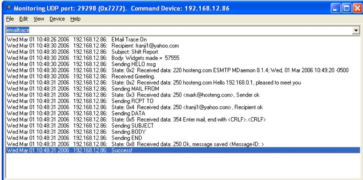
The screenshot shows a window titled "Monitoring UDP port: 29298 (0x7272). Command Device: 192.168.12.86". The window contains a menu bar (File, Edit, View, Device, Help) and a text area labeled "emailtrace". The text area displays the following SMTP trace:
