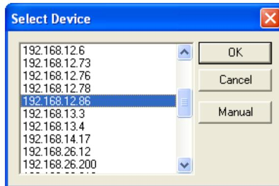
Choose the ECOM100's TCP/IP Address (in the example above it's 192.168.12.86), then hit the **OK** button. This will not do anything until you enter the proper command at the top of the SMTP Viewer Combo Box.
